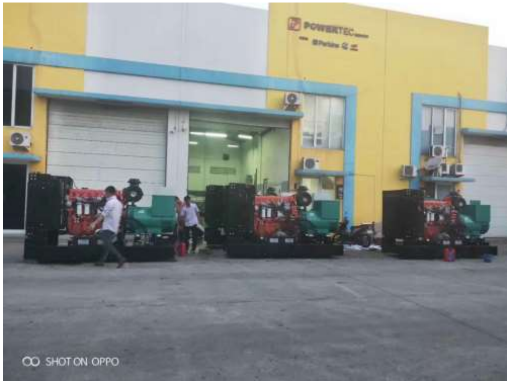
450kva genset for Jakarta-bandung high speed train project
