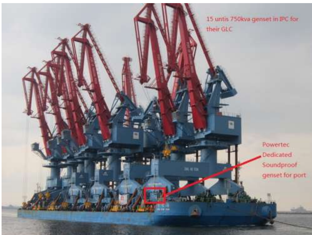
750kva Genset for GLC of Pelindo 2
